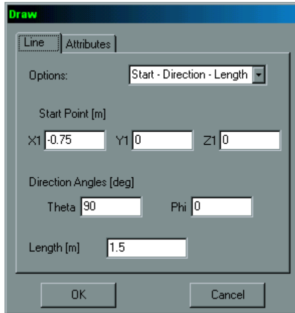
Fig. 3.3: "Line" page in the "Draw" dialog box for the wire "Line". "Start - Direction - Length" option.
